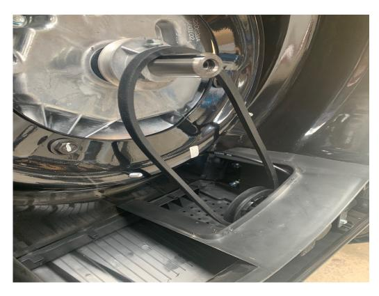
**REFIT BELT ONTO BOTH PLULLEYS**
