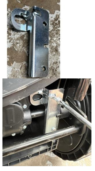
FIT THE NEW AXLE RETAINER PLATE AND SECURE WITH THE SCREWS FROM THE ORIGINAL
