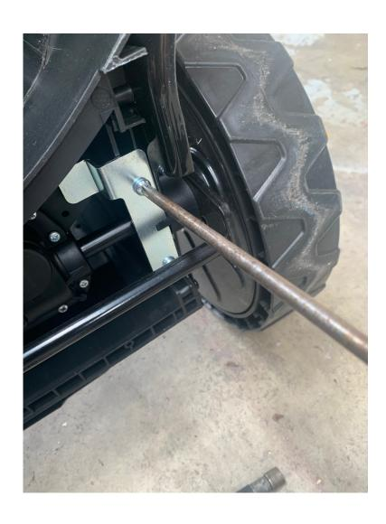
UNDO TWO PHILLIPS HEAD SCREWS ON THE AXLE RETAINER PLATE AND REMOVE AND DISCARD, KEEP THE SCREWS
