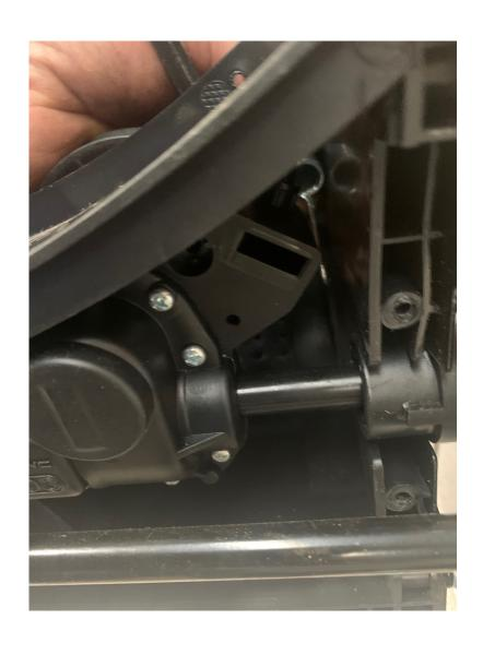
POSITION THE SPRING SO AS IT IS IS ACCESSIBLE TO HOLD WITH A PAIR OF LONG NOSED PLIERS
