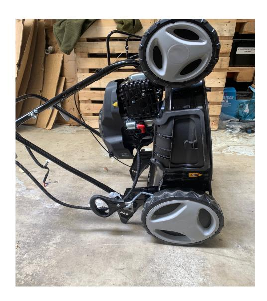
LIFT THE FRONT OF THE MOWER AND TILT BACK TO REST ON THE REAR WHEELS
