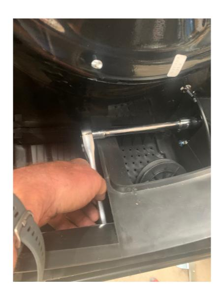
FIT NUT 1 SUPPLIED TO SECURE REPLACEMENT BOLT – FULLY TIGHTEN
