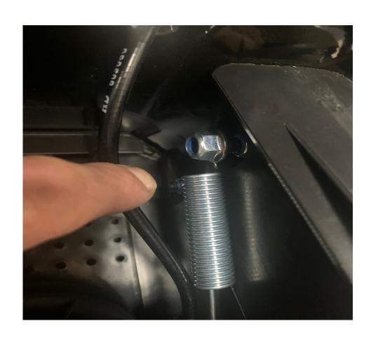
FULLY TIGHTEN THE SPRING RETAINING BOLT
