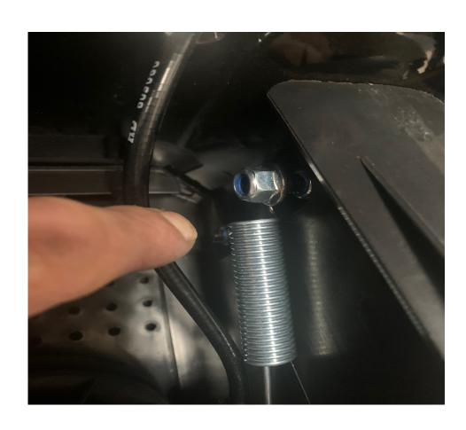
FIT NUT 2 LOOSELY TO BOLT TO HOLD SPRING IN PLACE
