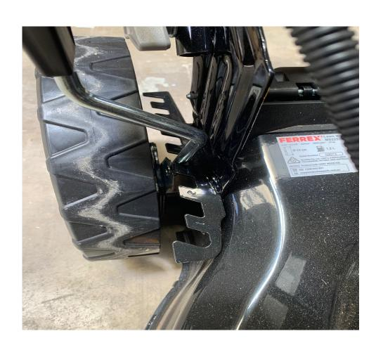
MOVE THE HEIGHT ADJUSTMENT HANDLES TO THE # 4 SLOT
