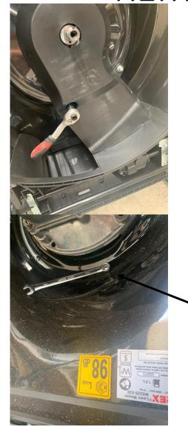
UNDO TWO 10MM NUTS HIGHER UP ON THE BELT COVER, USING A LONG SOCKET WILL MAKE THIS EASIER. THE HEAD OF THE BOLTS ON THE OTHER SIDE OF THE DECK ARE 8MM
