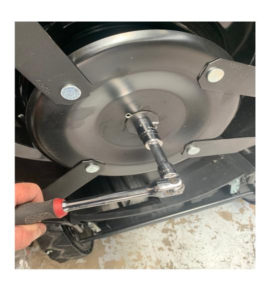
WITH A 17MM SOCKET OR SPANNER UNDO THE BOLT IN THE CENTRE OF THE BLADE DISC – ANTICLOCKWISE
