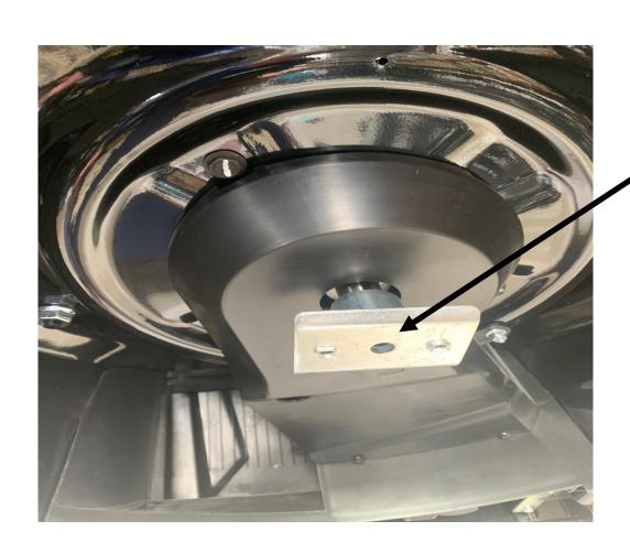
REMOVE THE BLADE DISC AND DISC SUPPORT PLATE
