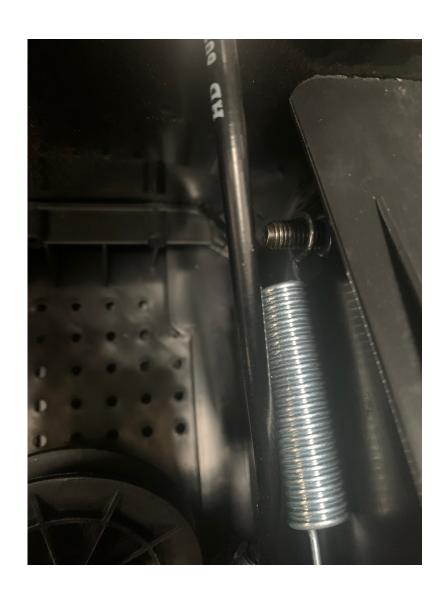
FIT SPRING TO BOLT USING CLOSED LOOP AS SHOWN
