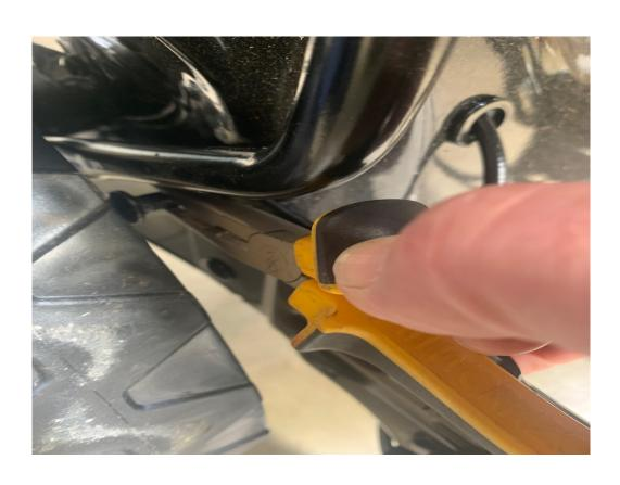
COMPLETELY REMOVE THE PREFITTED BOLT AND DISCARD
